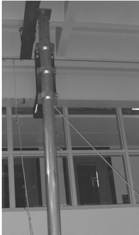
Figure 7-7 Macromanipulator Base Mounting
