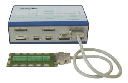
It is good practice to do some loop-back testing of an I/O option before connecting it to your real hardware under test. See Chapter 4, "xPC TargetBox I/O Options."
