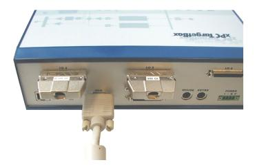
You are now ready to start the xPC TargetBox for self-testing. Because the xPC TargetBox does not have a power switch, the system starts to operate as soon as you plug the AC power cord into a wall outlet.
