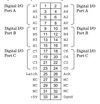
**Note** This connector does not use pins 35 to 50.
