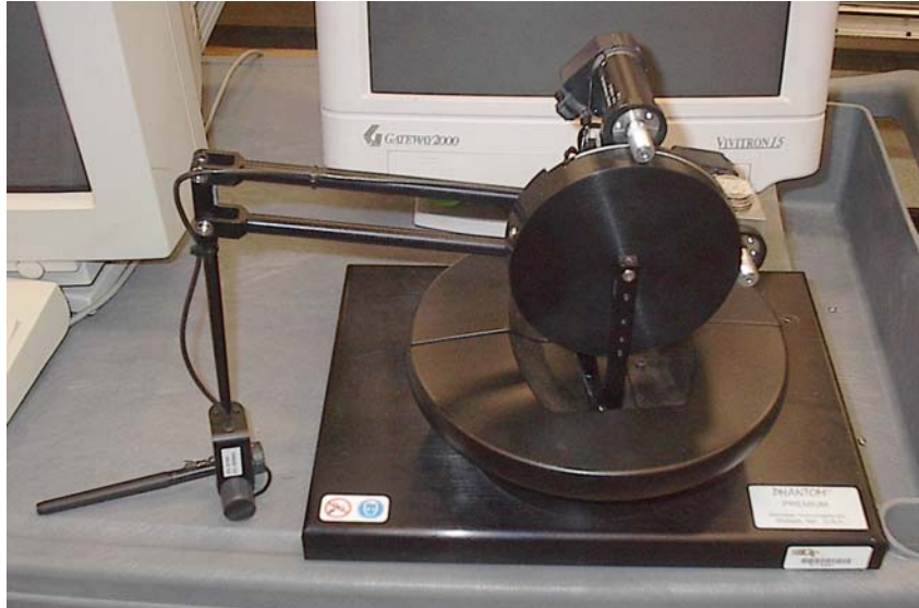
Figure 2: The PHANTOM Haptic User Interface
