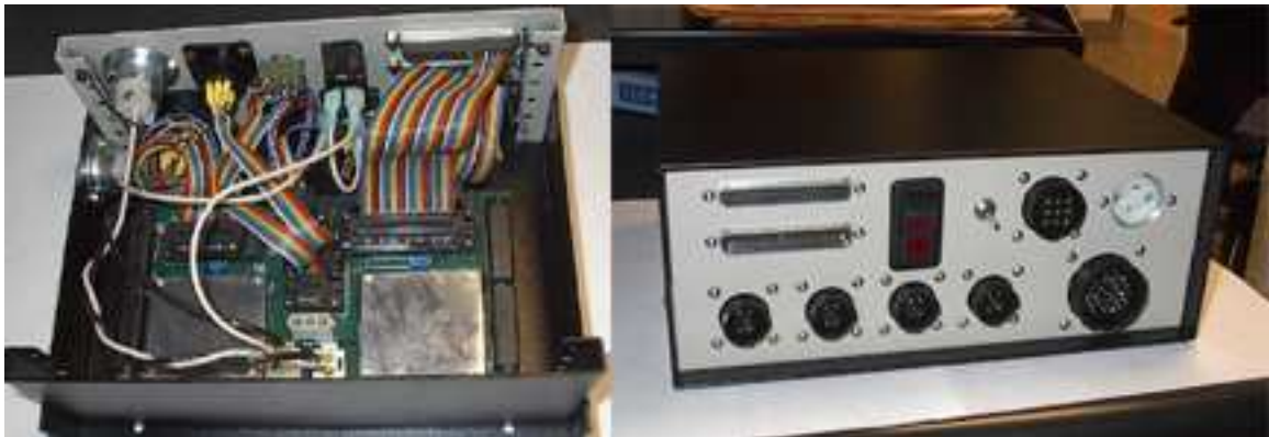
Figure 51: Power supply / signal junction box, assembled
