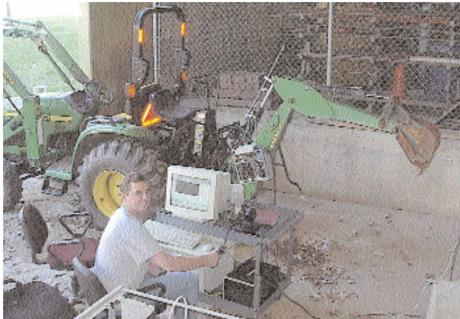
Haptic Backhoe initial trials — with student team leader Joe Frankel — focus on developing heavy equipment interfaces for the "Nintendo Generation."
