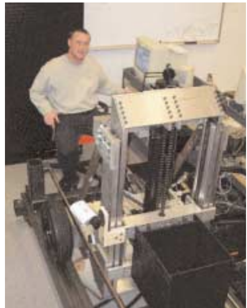
HAL, the laboratory forklift imitation, is shown with Ph.D. student Matthew Kontz. Matt and MS student Jonathan Beckwith are documenting the improvements possible with haptic controls.
